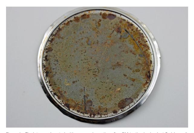
Figure 1 - Tinplate panel coated with an organic coating after OM testing in simulant B, 1 hour @  $130^{\circ}\text{C} + 10 \text{ days}$  @  $60^{\circ}\text{C}$
